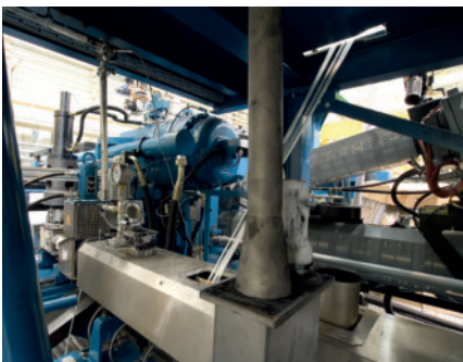
Extrusion system with the feed zone for the glass fiber rovings and the vacuum connection for degassing. The accumulator head for storing melt during injection is located at the front end of the barrel. The barrels of the injection units of the molding machine can be seen in the background
