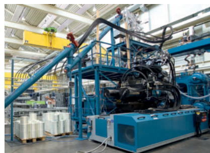
Close-up view of the two plasticating modules: at the left, the extrusion system with stand-alone conveying and metering equipment; at the right, the plasticating unit of the injection molding machine. This affords the opportunity to operate the latter independently from the compounder without any technical constraints whenever necessary
