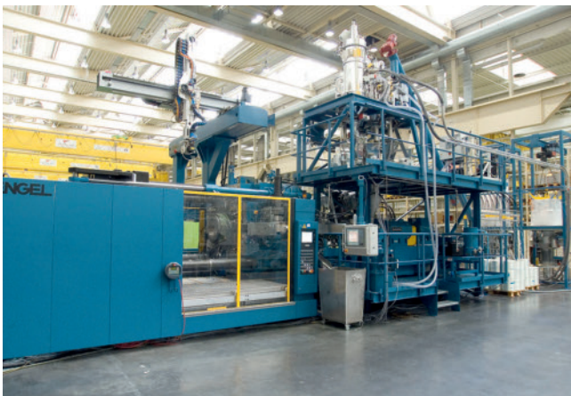
Injection molding combined with compounding: The modular concept for the system consisting of a standard, high-tonnage Duo Series injecting molding machine and a standard twin-screw extruder, including the equipment for material conveying and metering. An Engel ERC Series linear robot with the necessary peripherals is used for the handling of the parts
