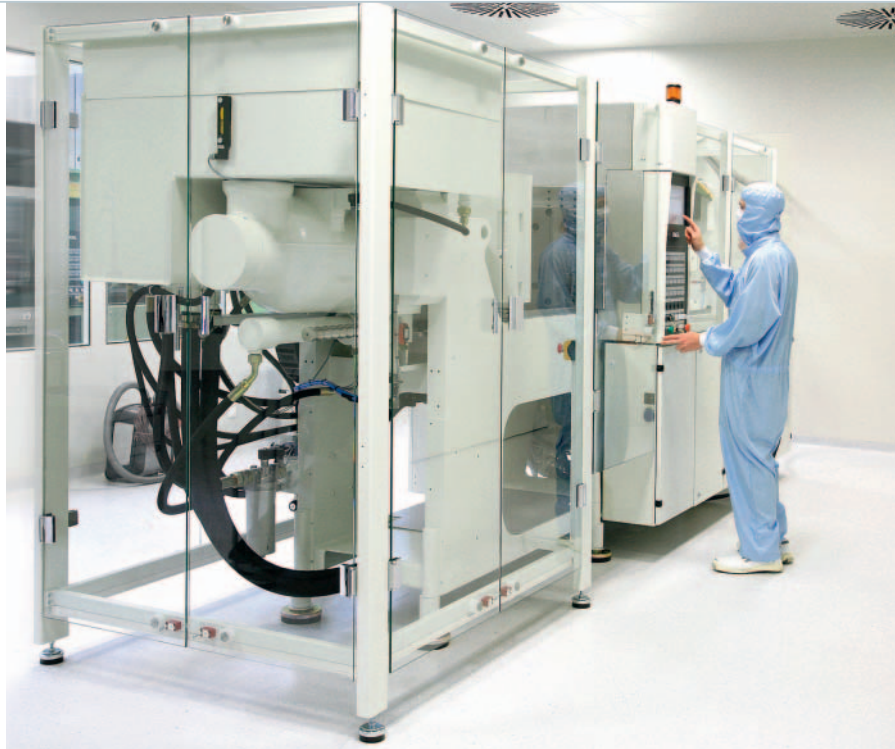
The specially adapted injection molder for cleanrooms integrates the two essential sector specific requirements in its philosophy: cleanliness and precision
