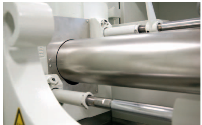
Fig. 5. The patented GMP barrel concept prevents emissions in the cleanroom
