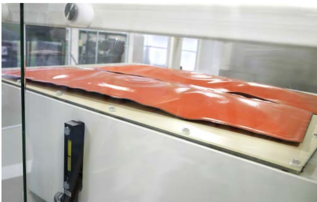
Fig. 4. Thanks to the closure of the tank with bellows, the entire hydraulic system works as a closed system
