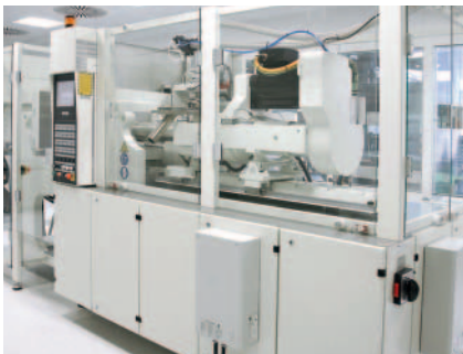
Fig. 6. The cladding made from glass and smooth profiles is easy to clean
