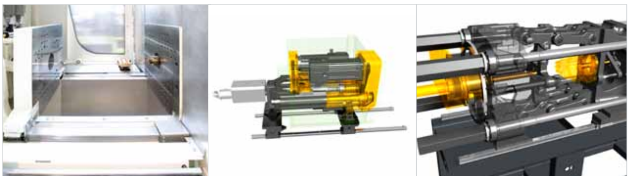
Completely greaseless clamping unit due to covered guides on the ENGEL victory
