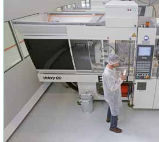
Satellite concept: the injection moulding machine is installed outside the clean rooms
