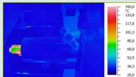
The thermal camera image shows it quite clearly: the patented GMP barrel extraction unit significantly reduces heat emission into the clean room.
